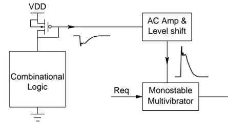
Fig. 2. Block diagram of the proposed completion detection system.
