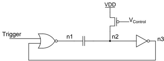
Fig. 6. Basic monostable multivibrator with variable resistor.
