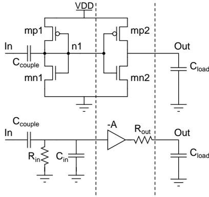
Fig. 4. Schematic and the small signal model of the AC-coupled amplifier used to amplify the detected signal.
