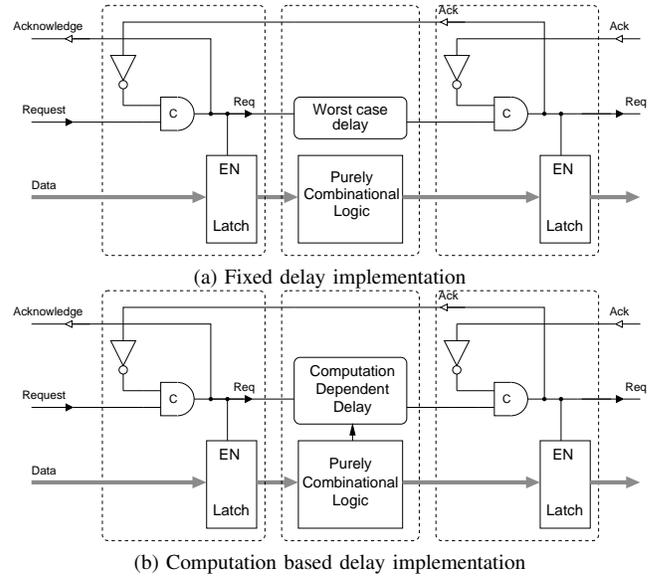
Fig. 1. 4-phase bundled data pipeline (After [6]).
