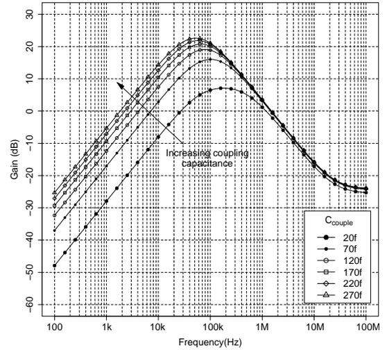
Fig. 5. Frequency domain response of the AC-coupled amplifier for multiple coupling capacitor values.
