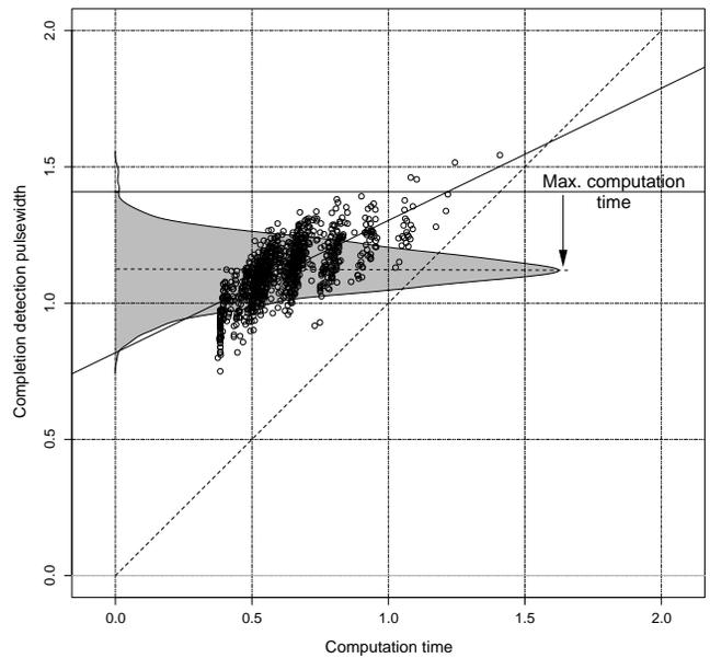
Fig. 7. Comparison of the actual computation time of the 8-bit adder and the monostable multivibrator response for randomly generated input vectors.
