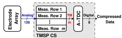
Figure 1. Proposed TMSP CS system high-level block diagram.
